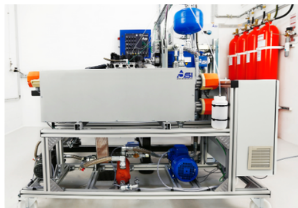
Oil conditioning unit with accurate temperature and flow control (coriolis flowmeter)
