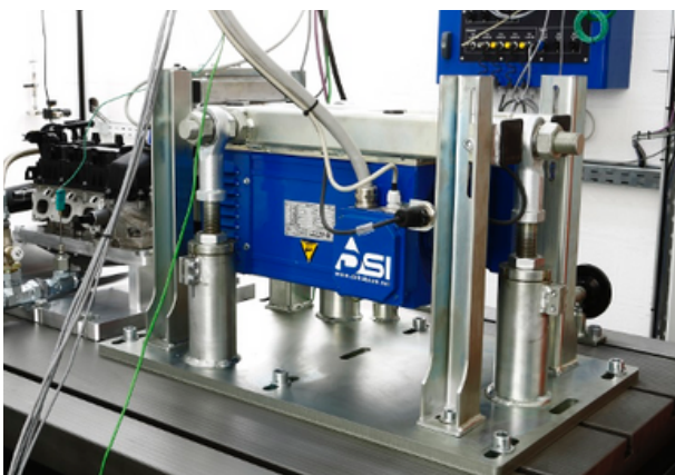
Cylinder head test rig – rear view - the electrical motor is installed on a platform with adjustable height
