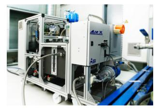
Our AIR-X equipment for real-time measurement of aeration levels in oil.
