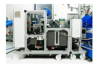
A **fluid conditioner** equipped with an aeration generator that covers aeration rates between 0 and up to 70%.
