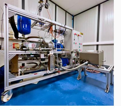
FLUCOIL is equipped with a range of smart probes to investigate oil quality during the aging process.
