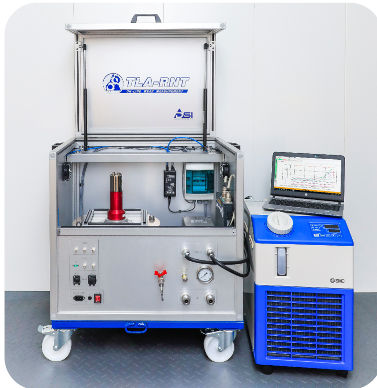
Figure 3 : TLA-RNT Chamber for Flow-through measurement
