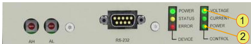
Fig. 23 Flashing LED with the sense function VOLTAGE LED -1- , POWER LED -2-
