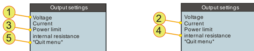
Fig. 81 Entry of the output settings – DISPLAY22
