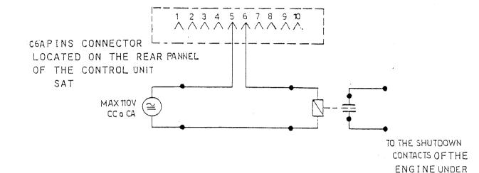
On pins 8,9,10 of C6A connector are available additional external alarms (lack of water pressure or water overtemperature). It is necessary to fit, on the water circuit, pressure and temperature switches and to connect the normally closed contacts. If either contact opens the respective led on the unit front panel lights up and the actuator goes immediately in the idle position and stays until the reset of the alarm condition.
