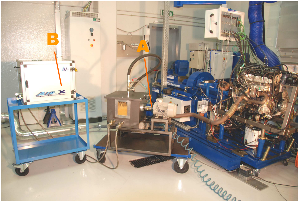
AIR-MIX equipment for supplying aerated oil to an I.C. engine, installed in a test cell
